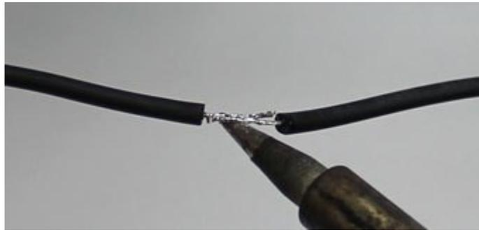
Figure 9: Soldering two wires.
