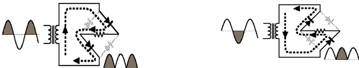
Figure 3: Both conduction paths through the load resistor
